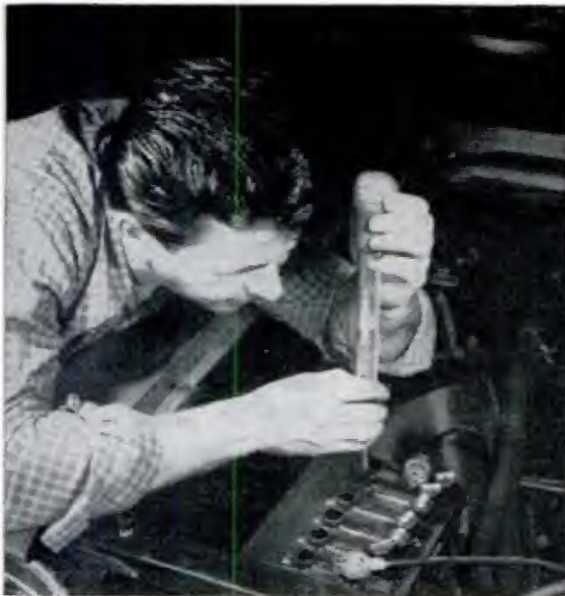
INEXPENSIVE HYDROMETER is used to check specific gravity of electrolyte which reveals state of charge
